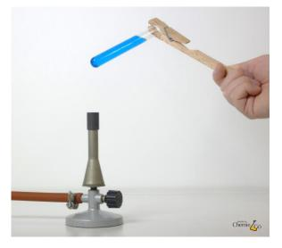
With the help of the test tube holder, a test tube can be heated over a Bunsen burner. To prevent boiling delay, the heating should be interrupted regularly. The opening of the test tube should always held towards the fume hood and away from the body.
