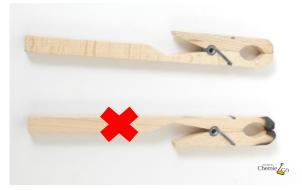
Furthermore, the test tube holder should not come in contact with the flame.
