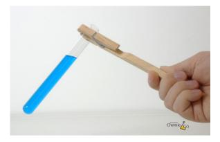
For safe handling in the lab, test tube holders (typically from wood) are used.
